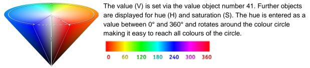
Values for saturation and intensity (darkness value) are set between 0 and 100%.100% mean complete saturation and full intensity.
