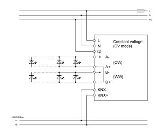
the outputs are automatically balanced based on the set brightnesses of channel A and B. The LEDs used must be compatible across the entire voltage range. The use of single wires is not permitted!
