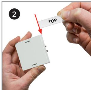
2 Insert the lever tool from above up to the first lock between the rocker and the lower part of the push-button. „TOP“ points to the front.
